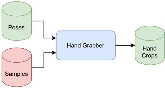
Fig. 2. Extraction of hand images (crops) from samples. The grabber is configurable. In this work we extract square regions enclosing all hand joints and resize them to  $70 \times 70$  pixels. Only hands with mean detection confidence higher than 0.4 are considered.
