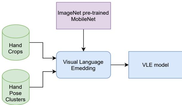
Fig. 4. We train the VLE model from the hand crops. Each crop has an assigned cluster (class) from the prior processing. The VLE is a MobileNet pre-trained on ImageNet and fine-tuned on our hand pose clusters.
