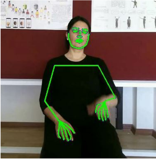
Fig. 2. Example of whole-body pose estimation on AUSL dataset. Note that this video is mirrored. The right hand of the signer is blurred due to its fast motion. Conventional hand detectors will fail in such cases. But whole-body pose estimation algorithm can still provide faithful keypoints estimation because it utilizes global information of the other body parts.
